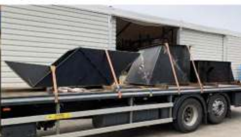
Chute sections to make up a full arrangement ready for site service installation.
