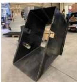
Ash hopper during fabrication as a direct replacement to an existing unit.
